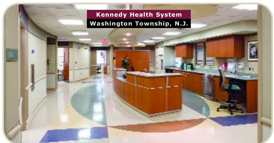
A strong flooring pattern can fulfill a wayfinding function by serving as a landmark that helps identify important areas to patients, visitors and staff.
