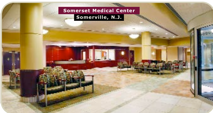
A floor pattern with darker hues of the same material can soften transitions and provide additional direction for patients, visitors and staff.
